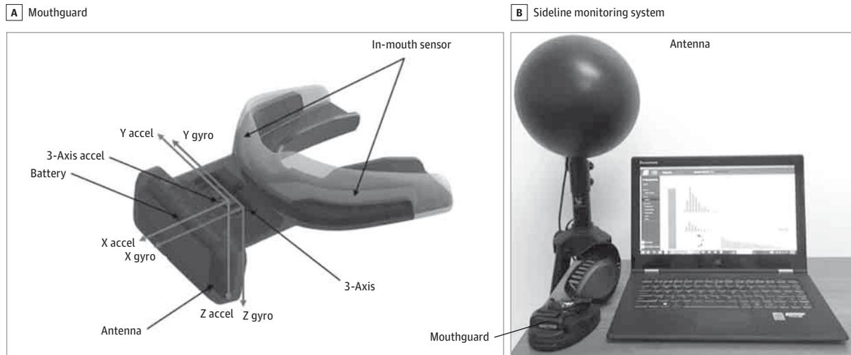
A. Triaxial accel senses linear acceleration and triaxial gyro senses angular acceleration. B. Sideline antenna receives impact data by radio transmission and store in the network server. Accel indicates accelerometer and gyro indicates gyroscope.
